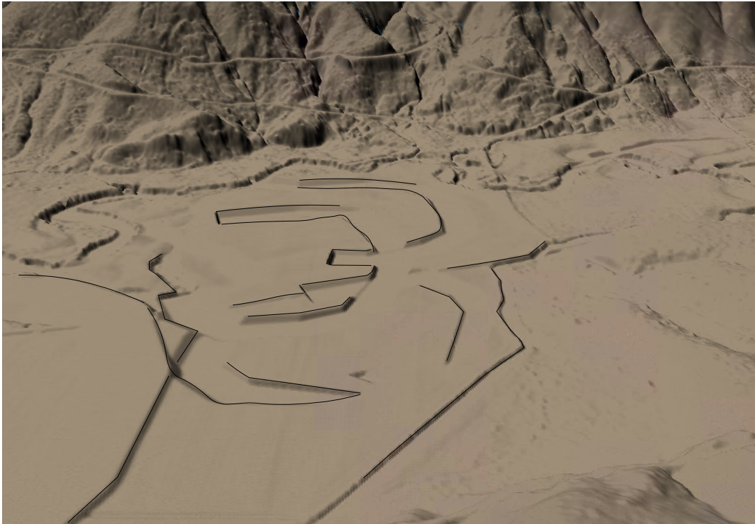
Figure 133a - Site Modification: Side Channels
