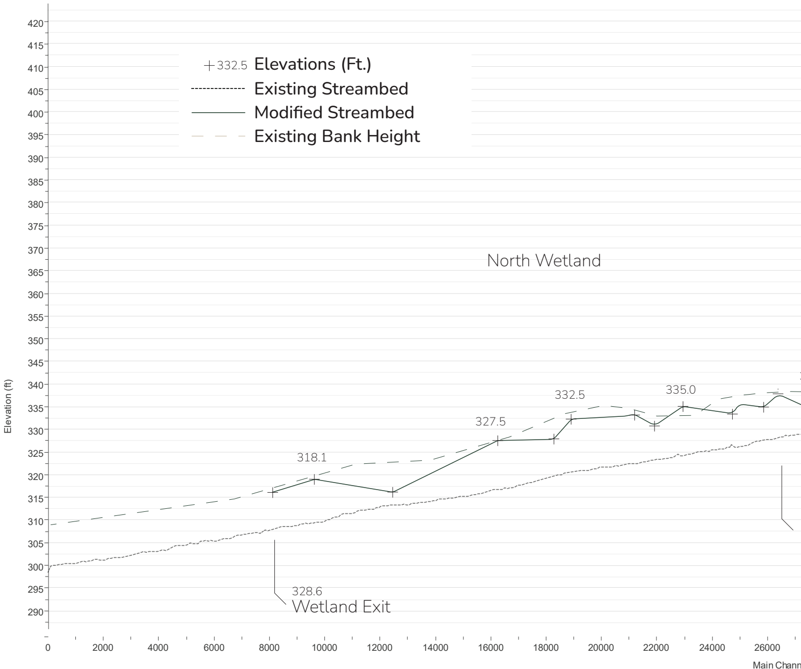
Figure 127- Elevation Profile with Modifications
