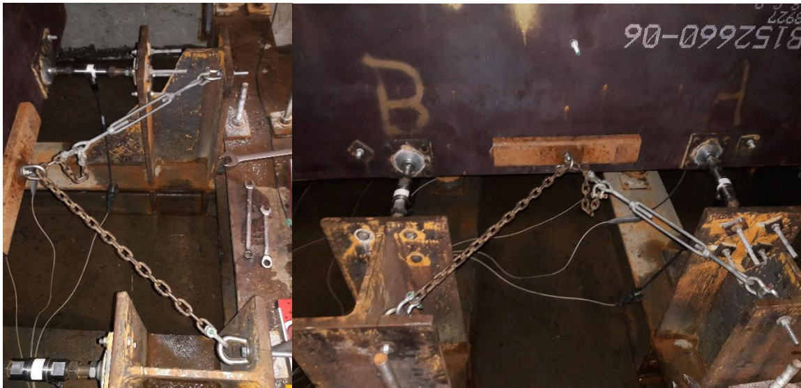
Figure 4-13: Stream-Wise Load Cells and Tensioning Chain
