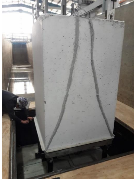
Figure 4-19: Strain Gauge Wires with Sealant Applied
