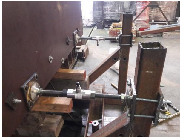
Figure 4-15: Transverse Load Cells
