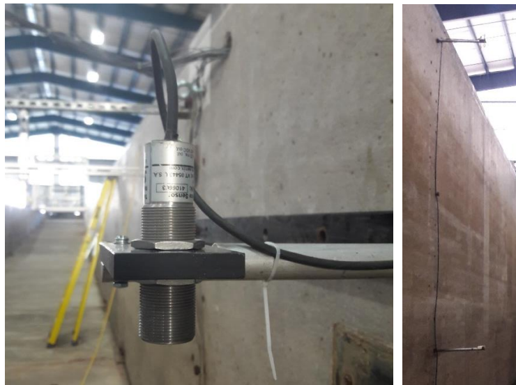
(a) Ultrasonic Wave Gauge (b) Wire Wave Gauge
