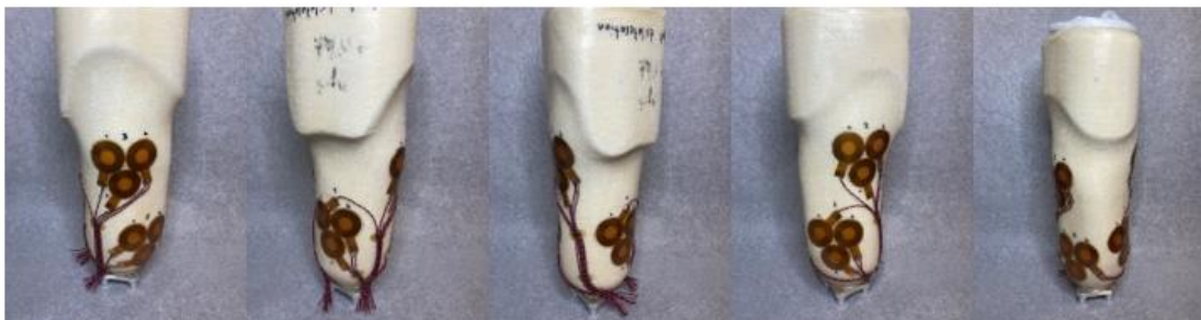
Figure 19: INTRAY sensor placement and wiring during the socket fabrication process for Participant One. Two arrays were wired into a single data collection board.
