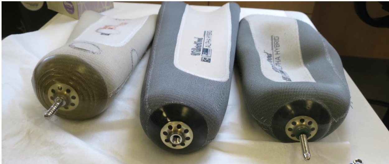
Figure 62: (left) Punch method investigational liner, (middle) new off the shelf liner that matched the practitioner prescribed liner, and (right) practitioner prescribed liner. Umbrella (plastic casing on the inferior edge) diameters are different between the investigational and practitioner prescribed liners.
