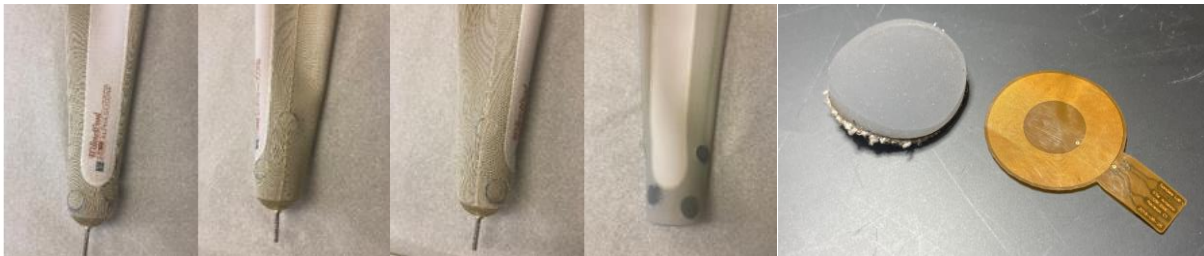
Figure 20: (a-c) The outside of an investigation liner fabricated using the punch method. (d) The inside of an investigation liner fabricated using the punch method. (e) A ferromagnetic-target liner punch compared to a single sensor from an INTARY, both having a diameter of 32mm.
