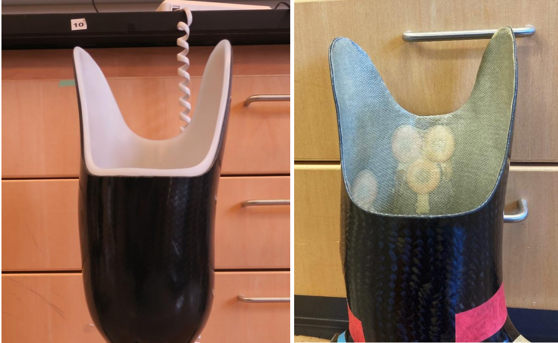
Figure 61: (a) Practitioner prescribed socket with flexible inner liner (white). (b) Investigational socket with the Patellar Tendon and Fibular Head INTRAY sensors visible. No flexible inner liner is in the investigational socket, and the brimline differences can be seen visually even though the two images were captures at different angles.
