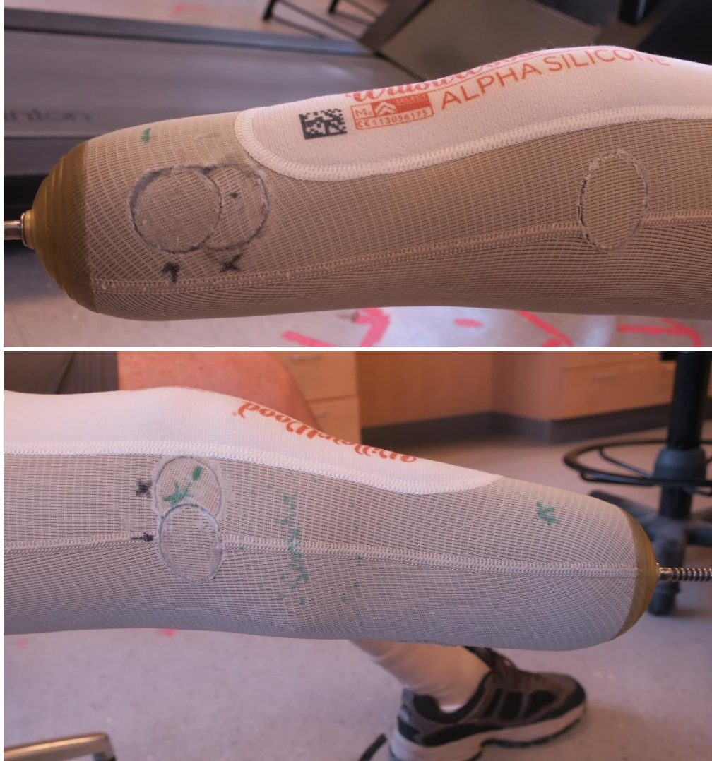
Figure 40: Participant Two's investigational liner fabricated with the punch method. The Anterior Distal and Fibular head sites required re-working so that the targets overlapped with the INTRAY sensors.
