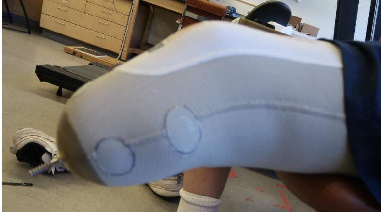
Figure 44: Participant Three's investigational liner fabricated with the punch method. The fibular head target is distorted because the liner is dramatically stretched over the participant's limb.
