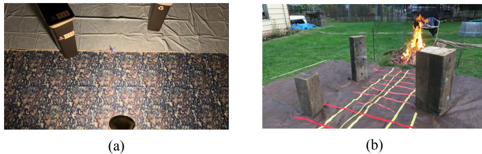
Figure 1.5: Experiment setup: (a) Arena for light source seeking, (b) Arena for temperature source seeking
