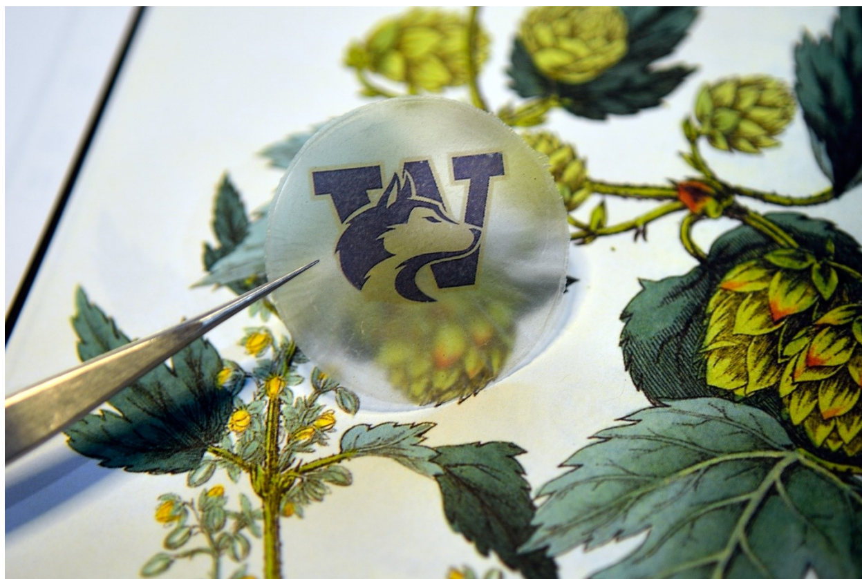
Figure 6.2. Film produced from 95% nanofibers and 5% PEOX, printed with a laser printer.
