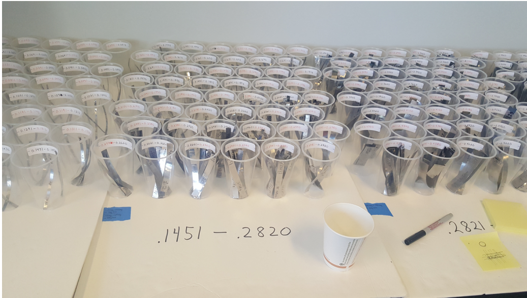
Figure 5.27: The image shows the manual histogram resulting from over 10,000 steel foils sorted by mass. The array of sorted foils helped to match the set of foil prescribed by the lamination optimization quickly.
