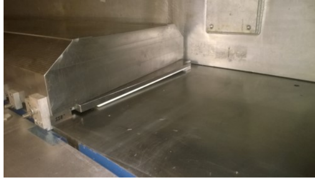
Figure 5.5: The image depicts a real wedge shim between the yoke in the pole piece. The protruding bolt on the left is used to adjust the edge shim radial position. The white spacer is used to ensure the wedge shim position is secure through power cycles of the storage magnet.
