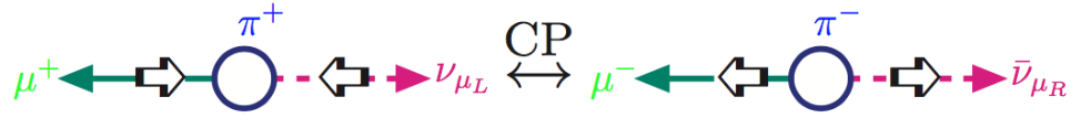
Figure 1.3: A diagram depicting pion decay in the rest frame. The spin vectors are shown in white and momentum vectors in color for the decay. Both the muon and the neutrino receive half the rest mass of the pion. The neutrino needs to have left-handed chirality, so both the neutrino and the muon are emitted with spin and momentum vectors anti-aligned. For the \pi^+ decay, the particles are emitted with right-handed chirality. Figure reproduced from reference [18].
