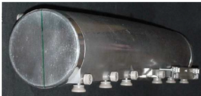
Figure 3.9: An image of the trolley module itself. The trolley rides along a rail system inside the vacuum chambers. It travels through the muon storage volume.
