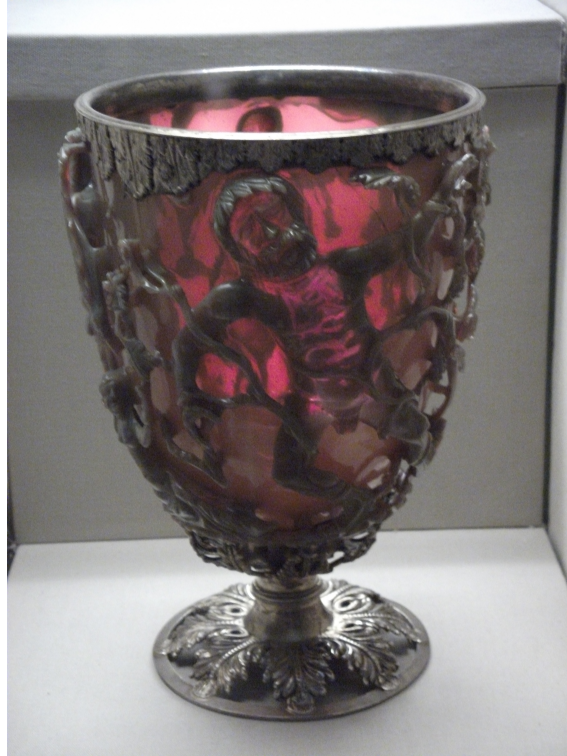
Figure 1.1: The Lycurgus cup contains plasmon-supporting silver and gold nanoparticles that cause it to appear green in reflection and red in transmission. Photo credit: Johnbod.
