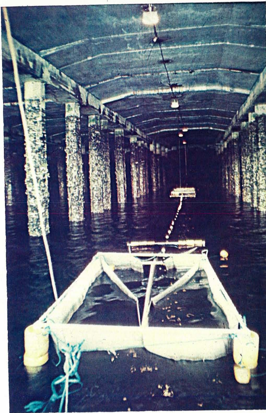
Plate I. Artificial light fixtures over juvenile salmonid trap array under the Terminal Four pier.
