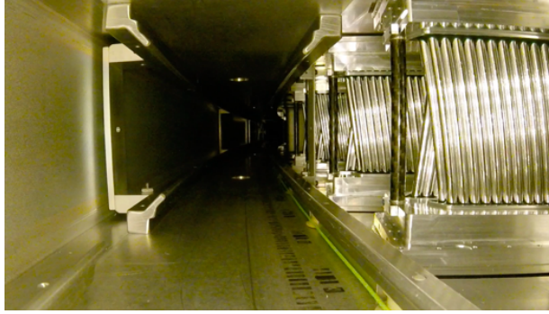
Figure 2.20: Photograph of a straw tracking detector taken from inside the vacuum chamber. The stored beam would be located at the center of the image. As stored muons decay into positrons, their tracks are measured in tracking detectors, allowing for their momentum and decay position to be reconstructed.
