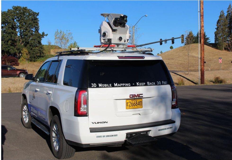
Figure 1.1. Mobile lidar system (Leica Pegasus:Two) owned and operated by Oregon DOT.
