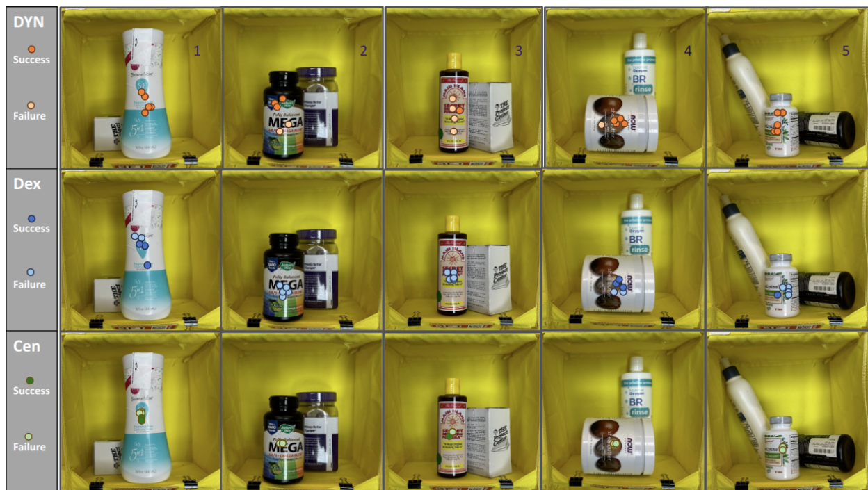
Figure 6.5: Real-world adversarial evaluation with five grasp points for each configuration: DYNAMO GRASP (our method), DexNet, and Centroid. The color-coded points represent the suggested grasp points success and failure from various algorithms. The successfully identified grasp points are marked by the color along the label “success” and “failure”.
