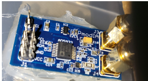
Figure 3.6: AD5933-based PIMODIA breakout board. Pins on the left are connected to Teensy 4.0, and coax cables on the right connected to the electrodes.
