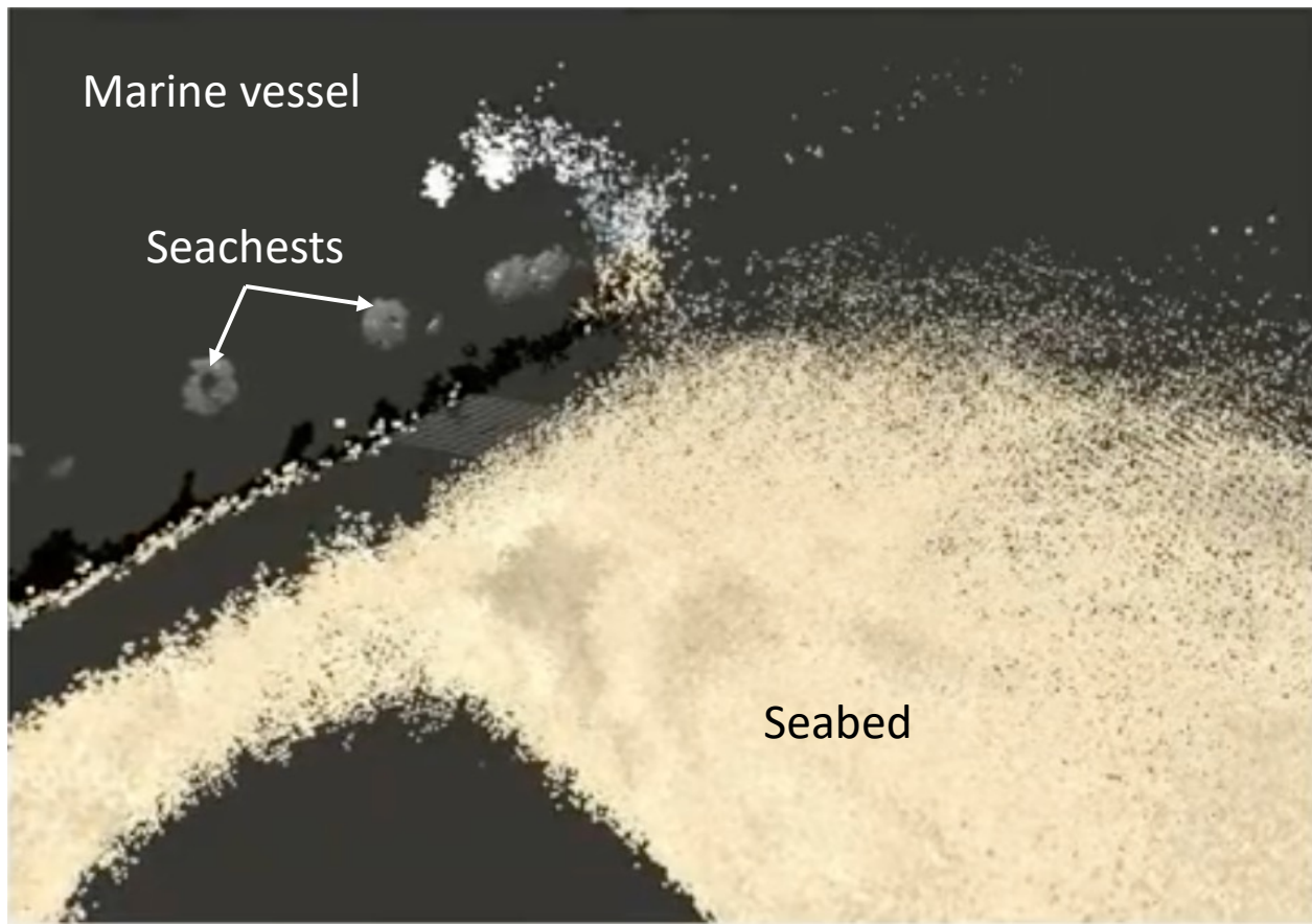
Figure 3.2: Partial map of an underwater environment generated by a BlueROV.
