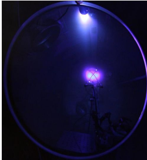
Figure 2.2: RMF magnetoshell tech demo. The magnetoshell is near the center while the MPD thruster plume is seen at top [14].
