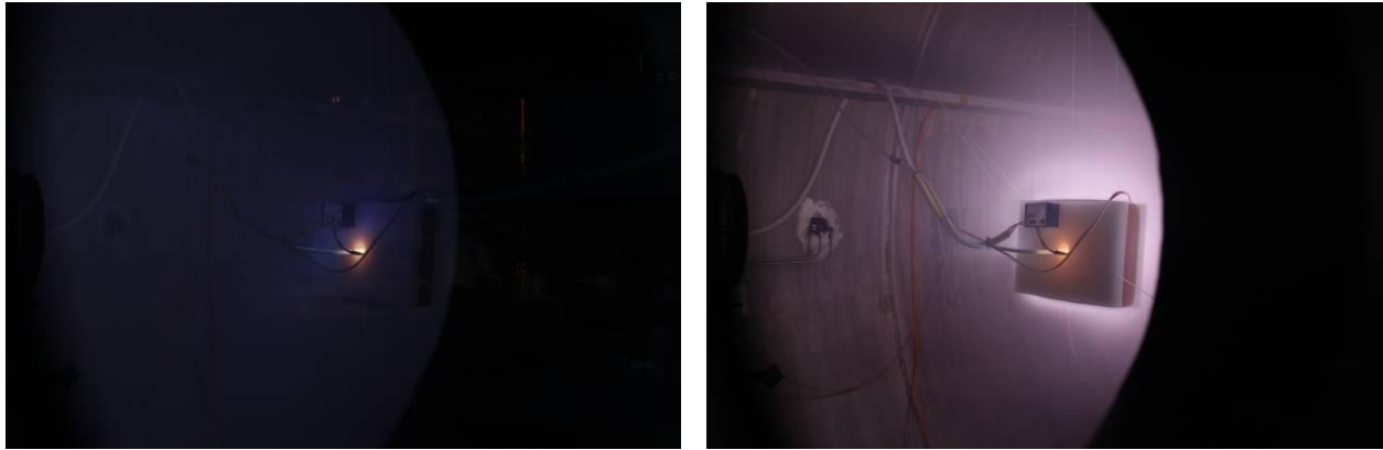
Figure 2.3: Mock 6U CubeSat with RF plasma injection at its center operating with Argon at 200 sccm, 300 W RF power, and B_0 = 0 Gauss (left) and 172 Gauss (right) [20].
