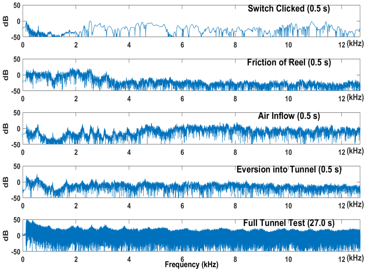
Figure 2.12: Audio FFTs of sound samples of isolated experiment components (0 to 12 kHz). Sounds are Switch Clicked , Friction of Reel , Air Inflow , Eversion into Tunnel , and a full tunnel test with all four transitions.
