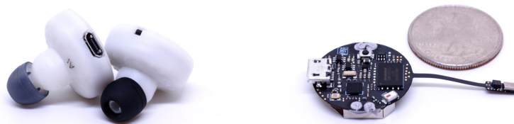
Figure 5.2: ClearBuds hardware inside 3D-printed enclosure and when placed beside a quarter.
