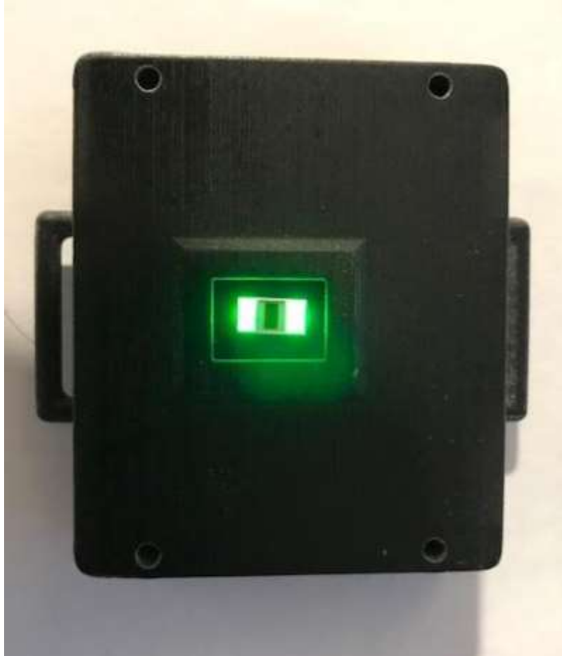
Figure 45 Health watch PCB housing bottom, with Sensor Array SFH7070
