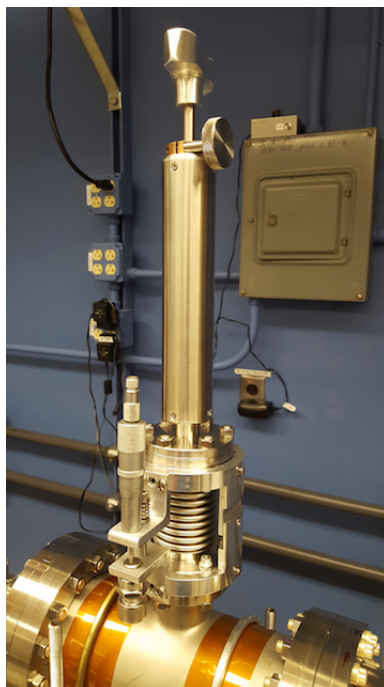
Figure 2.21: Photo of the translation stage. The translation stage is also shown on the left of Fig. 2.5. The translation stage allows vertical motion of the ion-detector. All the plastic parts on the translation stage have been replaced by aluminum parts such that the translation stage can be baked up to 200 °C.
