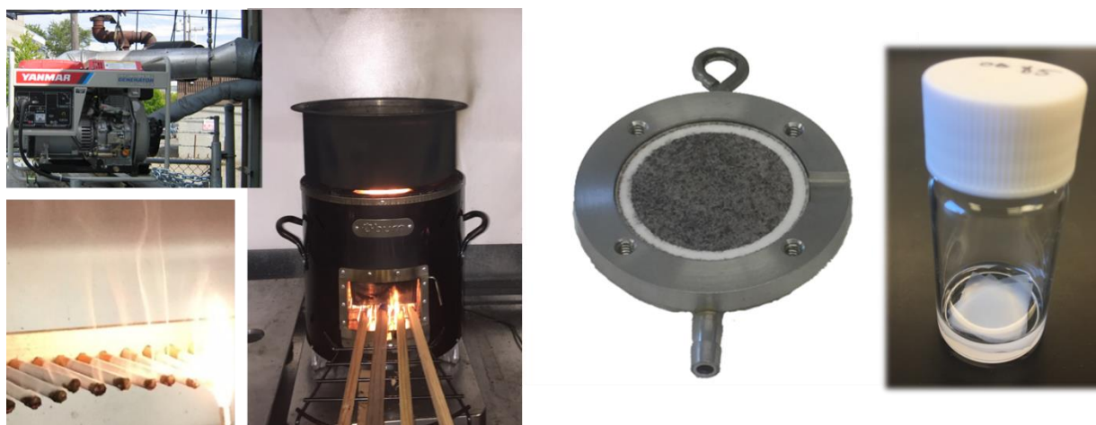
Figure 2.1: Photos of PM collection. From left to right: Laboratory sources of particulate matter (diesel exposure chamber, cigarettes, and clean cookstove), particulate matter collected on a PTFE filter, and PTFE filter in cyclohexane for extraction.
