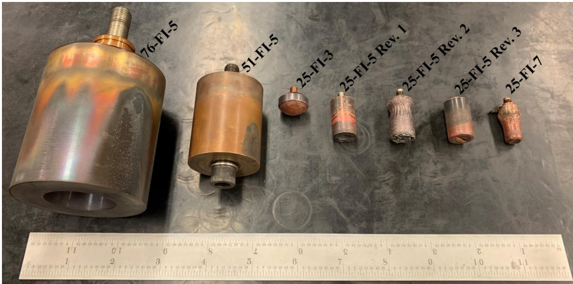
Figure 3.15: Post-fire condition of inner cores, including core failures.
