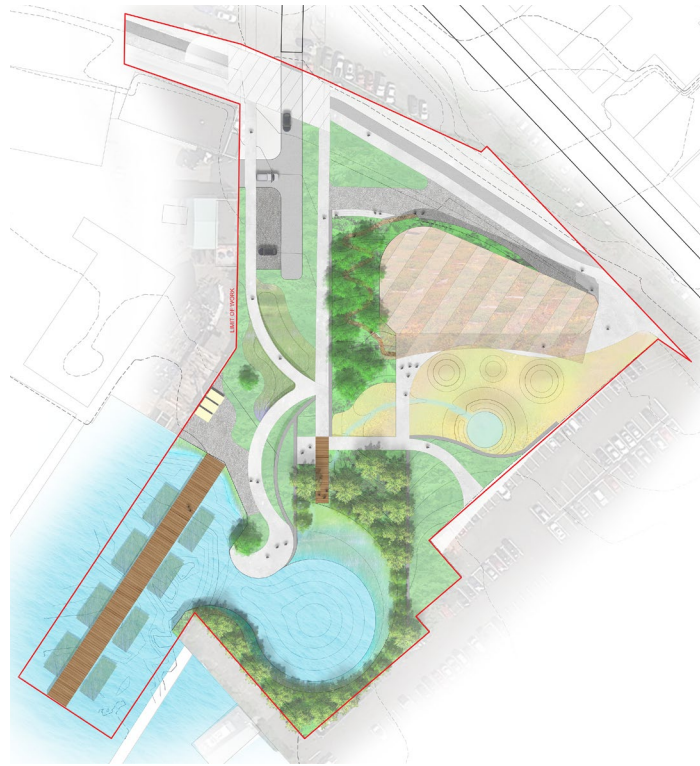
Figure 6.5: Site plan rendering of first schematic design. Emphasis in this iteration was placed on the habitat, by limiting human access to the shore and removing the existing building to create a salmon cove.
