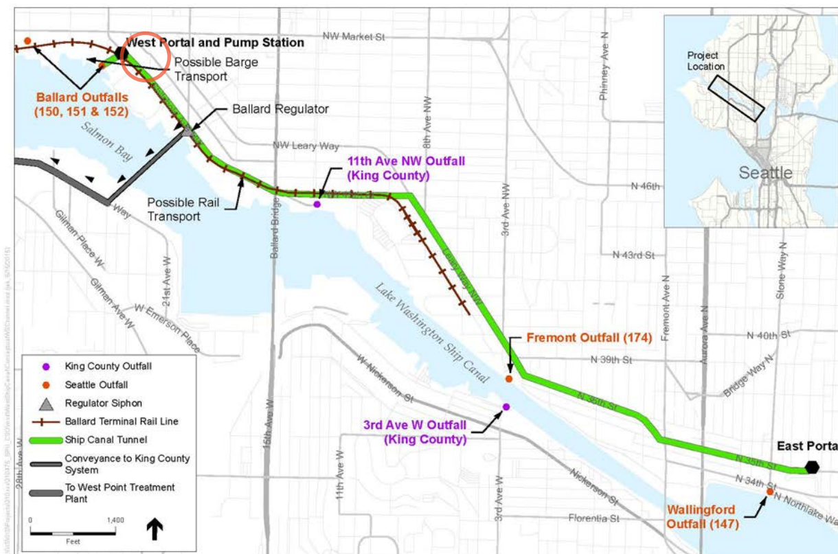
Figure 5.11: Proposed Ship Canal water quality tunnel project. Designed to help mitigate the occurrence combined sewer overflows by adding extra capacity to the sewer system for heavy storm events. The 24th Ave NW street end is site of the West Portal and Pump Station indicated on the map (circled in red). (Credit: Seattle Public Utilities).
