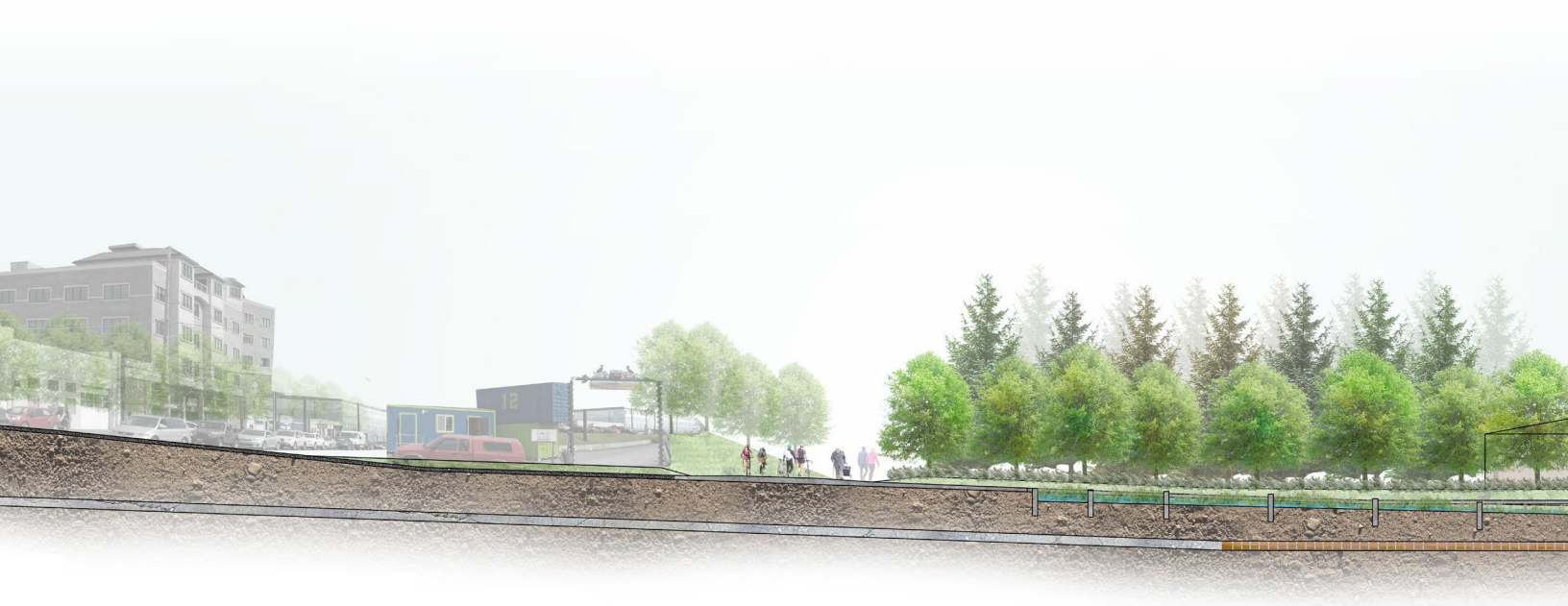
Figure 6.19: Section at Burke-Gilman Trail extension showing biofiltration swale and access drive to Pacific Fishmen's Shipyard.
