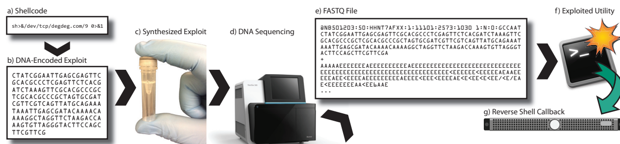
Figure 2.3: Our working exploit pipeline
