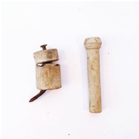
Knob and tube electrical insulators.
