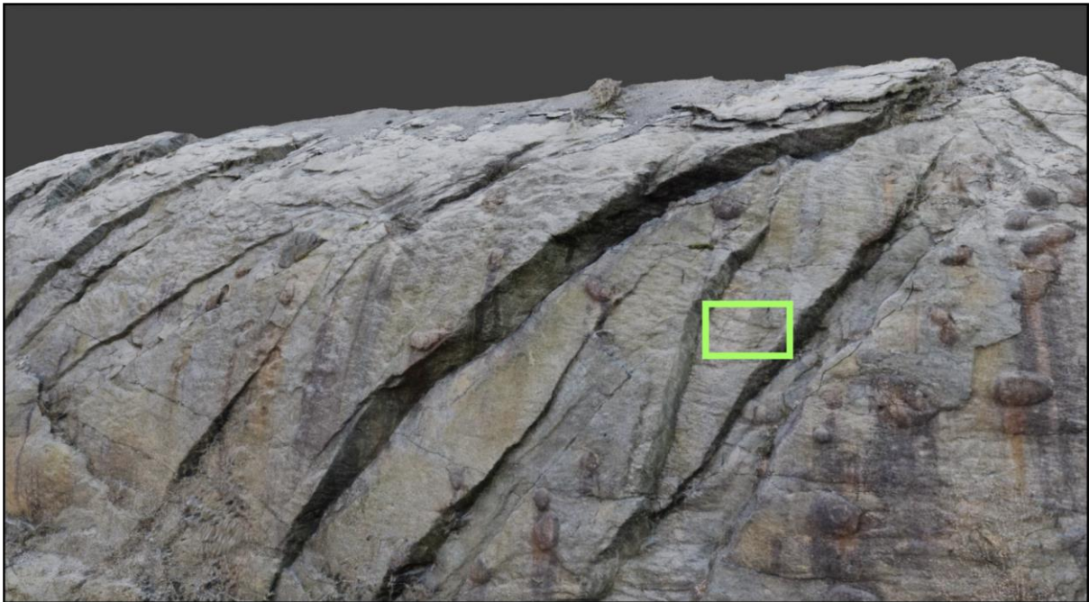
Fig. 5-9: Some features are only represented by the model's color data within the texture. Top) This shaded polygonal model was useful in determining contacts between fault surfaces and bedding. Yellow box does not include small horizontally oriented faults. Bottom) This is the same view of the model but textured. Yellow box includes small horizontally oriented faults. There are smaller faults represented in these color data that are not three-dimensionally represented by the polygons in the mesh data.
