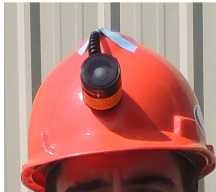
Figure 5: Sensor location on helmet.
