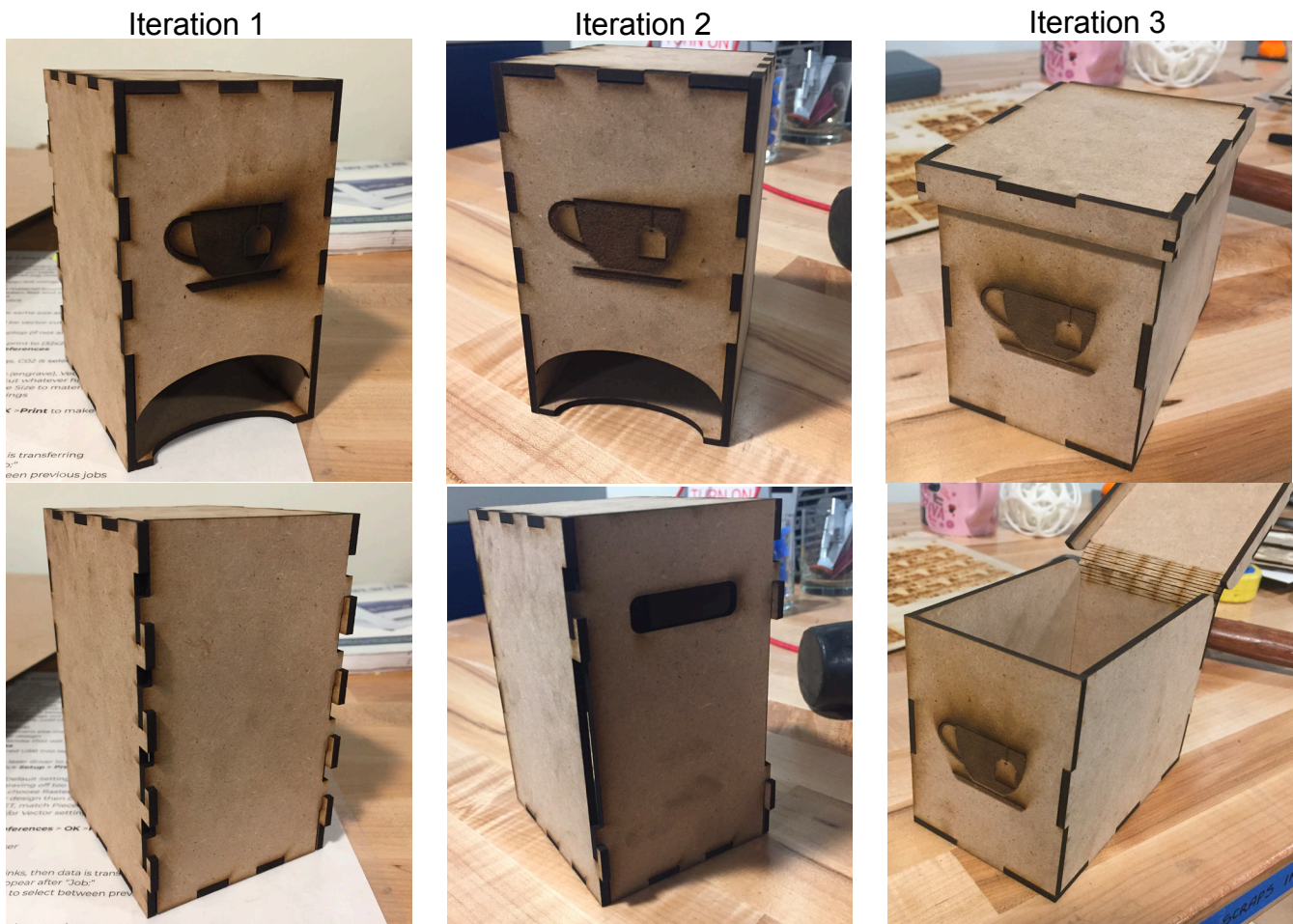
Figure 5_4: This figure depicts the three iterations of Karen's project, a box for holding and organizing tea bags. A front and back view of the first tea holder is pictured on the far left. This replicated the design from the tutorial pictured in Figure 5_3A. The middle two pictures show a front and back view of the second version of the tea box. Karen changed the speed and power settings on the laser to try to get a less charred appearance on the tea image. She also added a hole to the back to use as a handle and reduced the number of press-fit tabs for aesthetic reasons. A closed and open view of the final version can be seen on the far left. In this final version, Karen explored a different laser-cutting technique called a "living hinge." The technique creates flexible sections in a material by cutting specific patterns of holes.
