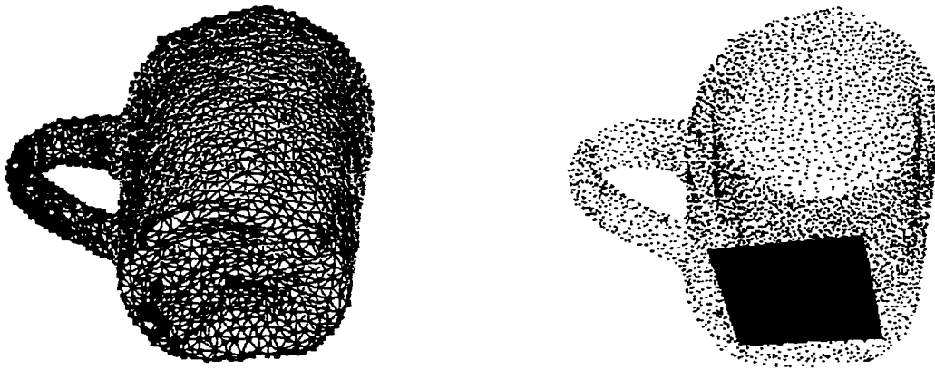
Figure 4.6: Bottom view of working sets for coffee cup mesh shown in Figure 4.2a. There is one PLANAR working set. Plane shape-type fit to the PLANAR working set. The plane is square for display purposes only; no assumptions are made regarding its shape.
