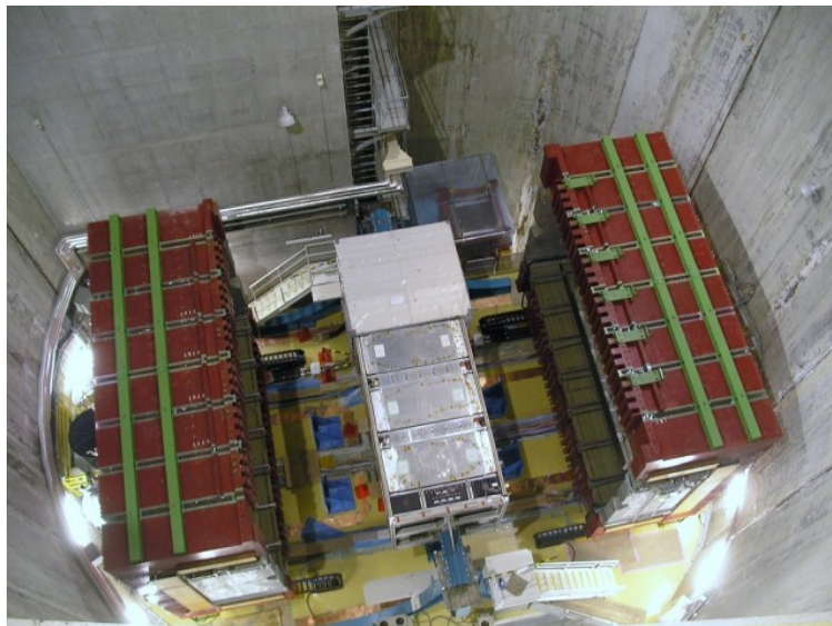
Figure 3.2: Picture of ND280-OA from above with the magnet open. The neutrino beam starts from the top of the pictures and moves towards the bottom of the picture.
