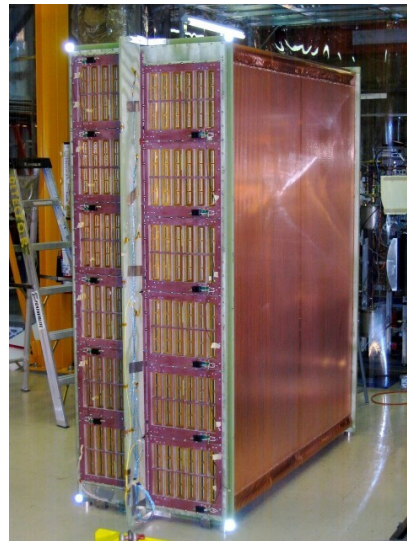
(b) Photograph of the inner box of a TPC.
