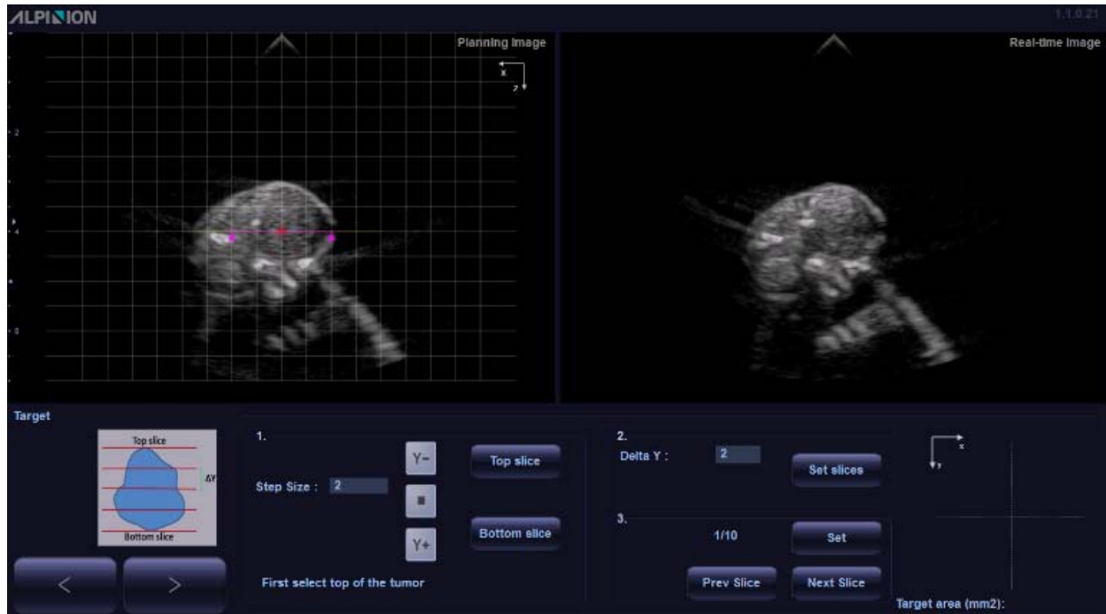
Figure 3.3 An example of user interface on defining treatment width on each the transverse slice of the tumor. The mouse was moved up and down at a step size of 1 mm along the vertical axis (head to tail direction). The positions of top slice and the bottom slice were determined by experienced sonographer and were recorded by the treatment planning program. The length between top and bottom slices was divided into a number of slices at a separation of 1 mm. The widths of the each slice can be individually determined to avoid collateral damage to other organs.
