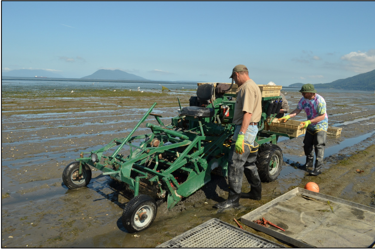
The modified tulip bulb harvester used at Chuckanut Shellfish Farm to harvest Manila clams. Photo courtesy of Daniel Cheney, Pacific Shellfish Institute. 2012.
