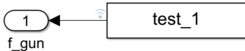
Figure 56: Rivet gun force block. It loads the generated gun force into the model.
