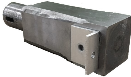
Figure 2: Steel bucking bar used during testing. It has typical bucking bar mass for fuselage riveting.
