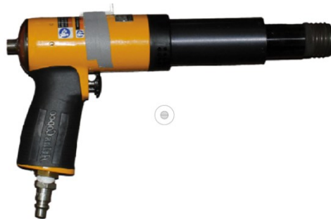
Figure 1: AC-10P rivet gun used during testing. It is the standard recoilless gun used at Boeing for fuselage riveting.
