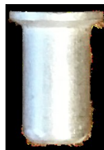
Figure 3: Rivet used during testing. It is the standard rivet used on an airplane's fuselage.
