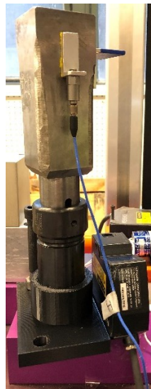
Figure 12: Bucking bar system setup for Simulink experiments.
