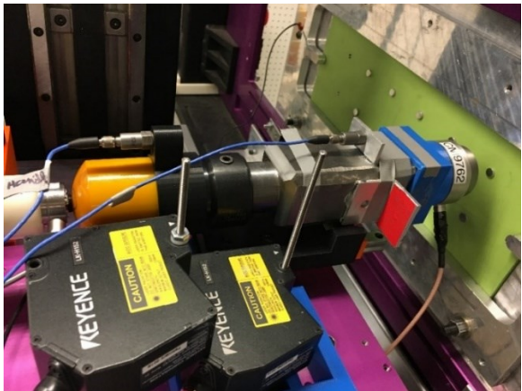
Figure 13: Bucking bar setup with a load cell attached to it and used to form the rivets. The load cell measured the force from the rivet to the bar.
