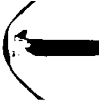
Figure 3.9: Binarized Mean field highlighting regions of high optical density in black. Bow shock location extraction achieved by taking the gradient of this image. (Test conditions: N_2 - N_2 , M_e = 3 , C_T = 4 , D_b = 1/8'' )
