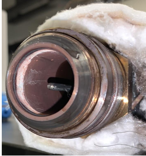
Figure S3: Shown here is the reactor with the Reactor Section TC (1") located in the center, as outlined in Figure 11. This is the most recent observation of rust within the reactor section after running the hydrogen peroxide experiments presented in this thesis.
