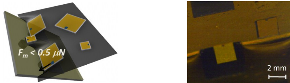
(b) violation 2: Parts in wrong orientation
