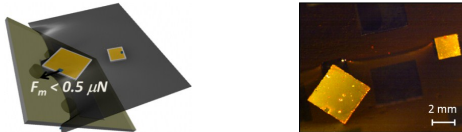
(a) violation 1: 4 mm parts on 2 mm binding sites.
