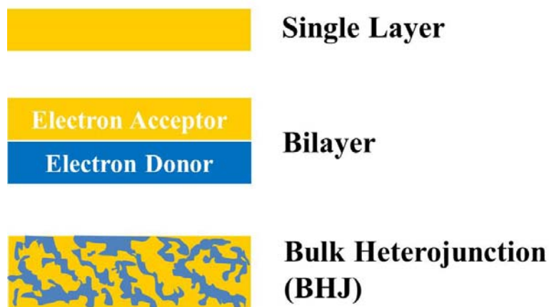
Figure 1.3 Schematic illustration of structure of active layer.
