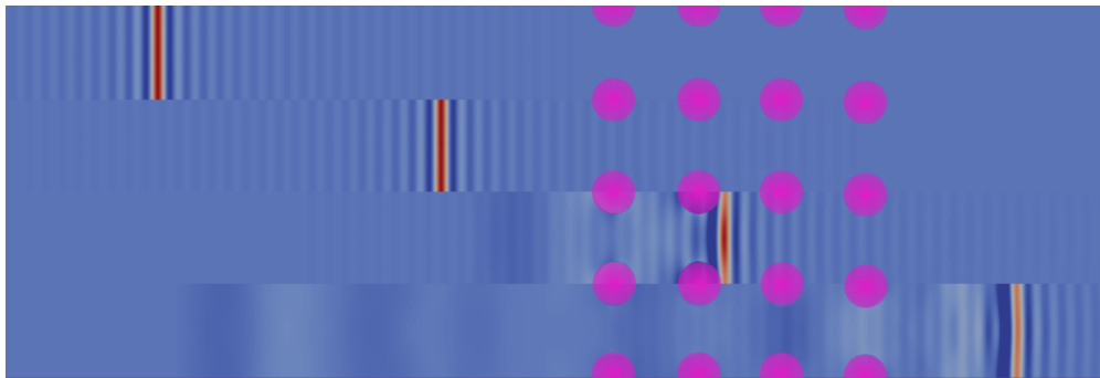
Figure 5.4: The simulation domain described in Fig. 5.3 overlaid with contours of E_y for four simulation times: in descending order, t = 0, 0.5, 1, and 1.5 ns. Locations of plasma columns are indicated in pink. The sinc waveform interacts with the plasma array causing certain wave lengths to be reflected, while most pass through unaffected.
