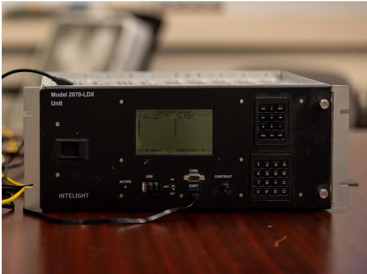
Figure 3-3 2070LDX traffic controller unit.
