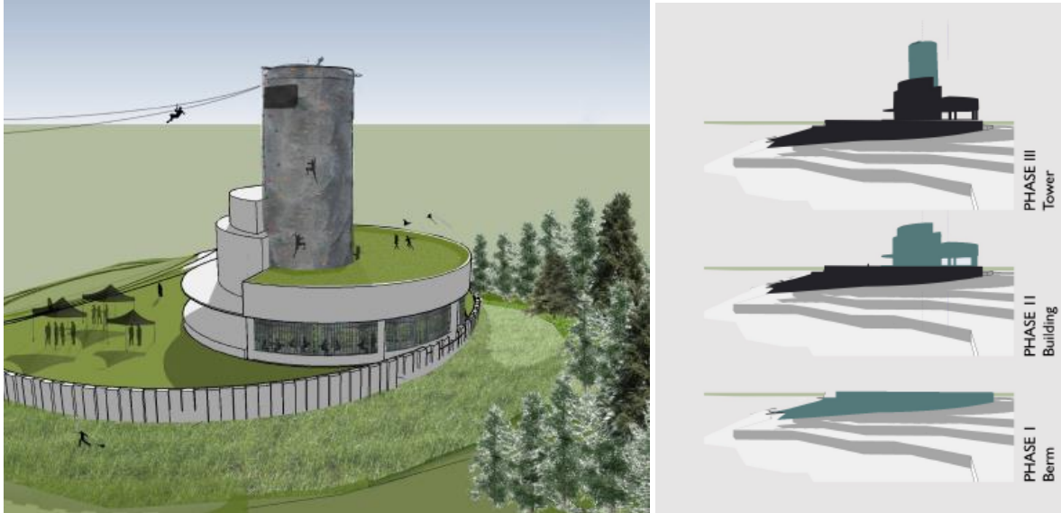
Figure 9. Conceptual image of a vertical evacuation structure as a recreational physical activity center, buildable in phases.
