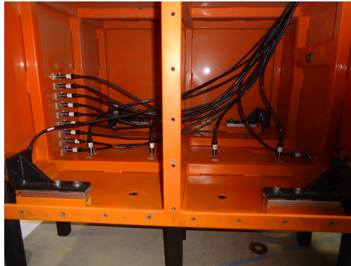
Figure 2.8: Typical Pressure Gauges Installation [2]
