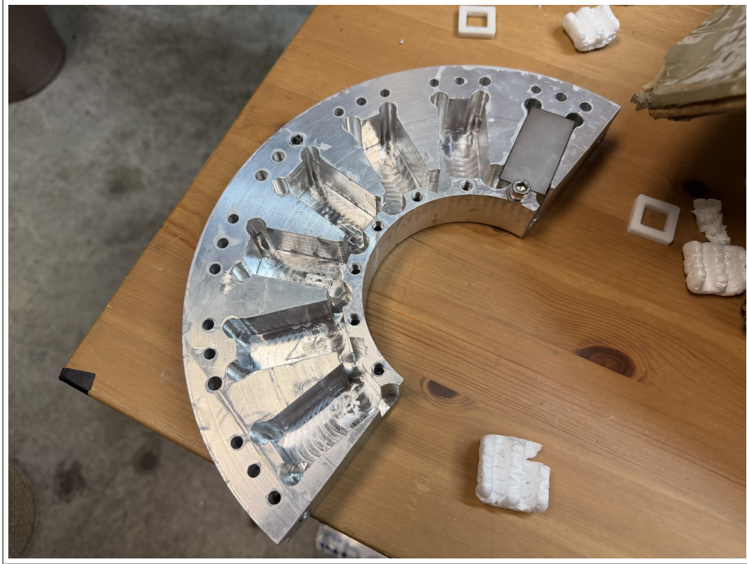
Figure 4.1: Machined aluminum permanent magnet enclosure containing the split-ring geometry and rectangular magnet-pocket layout.
