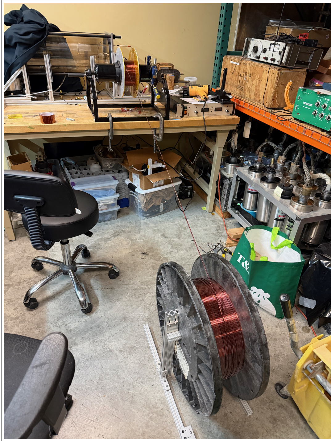
Figure 4.4: Spool stand and wire-feed setup used to support the large magnet-wire spool during solenoid winding.
