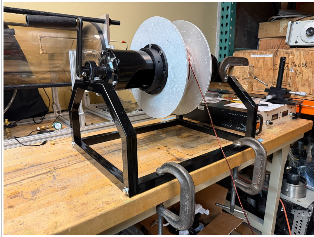
Figure 4.3: Winding jig used to control the mandrel, bearings, axle, ratchet interface, and wire feed during solenoid manufacturing.
