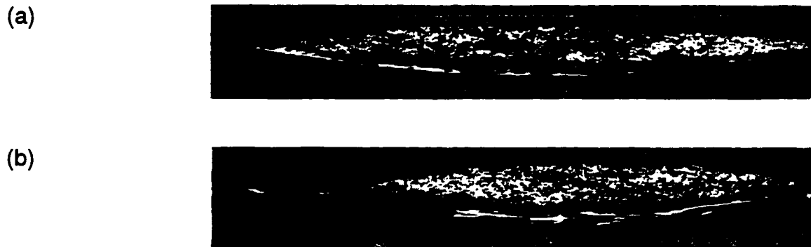
Figure 3.19 Optical photomicrographs of the cross-sections of experimental preregs manufactured with two impregnation rollers and a) no fabric tension and b) high fabric tension.
