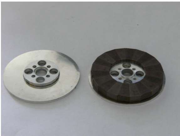
(c) Attractor spin-ring mounted with the centering-fixture aligning it with the compensator disk below the \mu -metal annulus.
