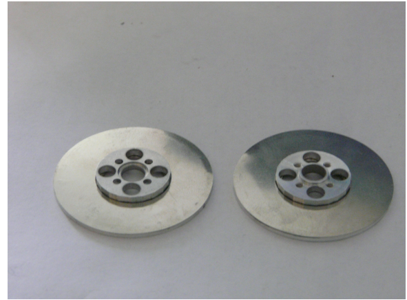
(b) \mu -metal annuli in position on the compensator disks.
