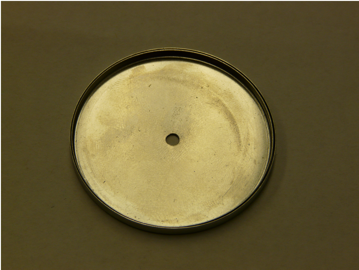
Figure 6.1: Photograph showing the top half of the Mark II pendulum cans, sitting nested inside one another.
