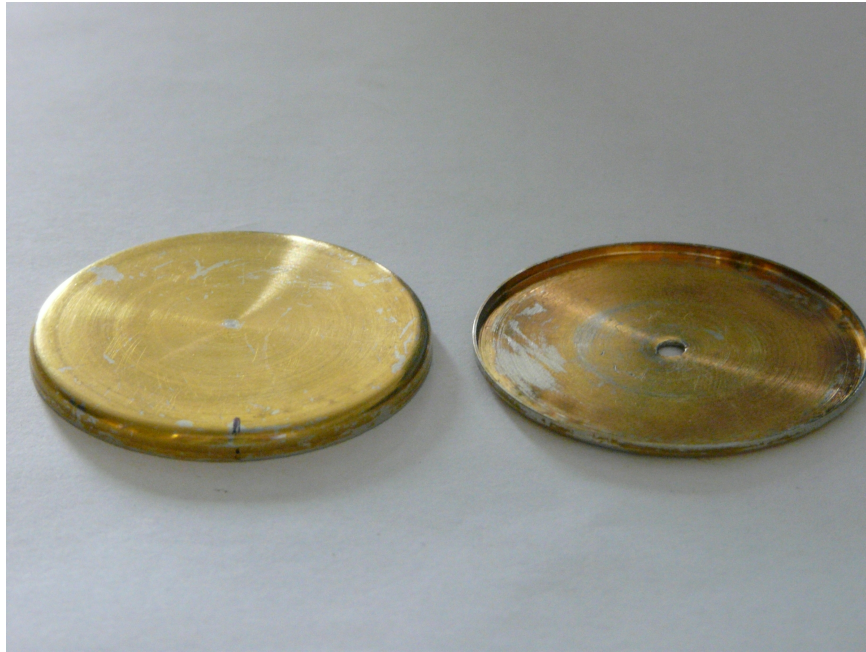
Figure 3.11: A photograph of the \mu -metal can which enclosed the pendulum active elements.
