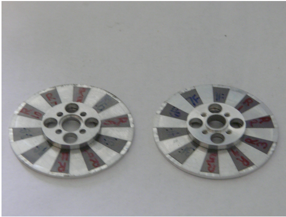
(a) Compensator disks with shims glued in and mounted on centering-fixtures.
