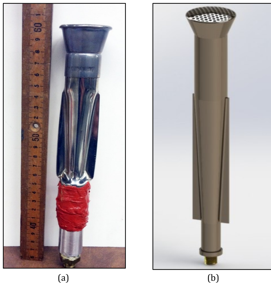
Figure 3.5: Side view of the Meker burner top as used in the experimental setup. (a) Actual Meker burner, (b) CAD model of the Meker burner.
