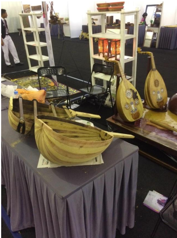
Figure 17: Gambus making demonstration at the Kuala Lumpur Craft Complex. Notice the strips of wood forming the bowl of the lute. 13 September 2015. Photo by Joseph Kinzer.
