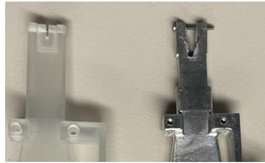
Figure 6 Clamping mechanism before and after post-machining modification. Aluminum version with gap deepened by post-machining to restore clamping compliance and reliable probe retention is shown on the right.
