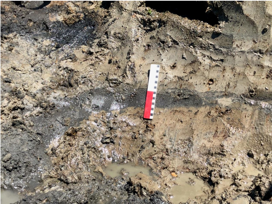
Figure 2.3 Paleoliquefaction. Remnants of sand ejecta from a sand boil along the Duwamish River in Seattle, Washington. Liquefied sand penetrated the non-liquefiable lower silt followed by deposition of the upper silt.
