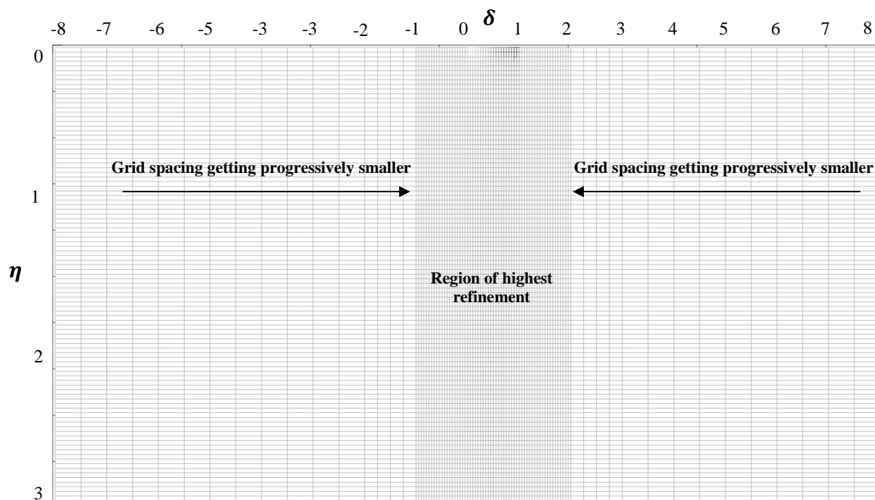
Figure 5.48. Grid used for mapping stresses with higher refinement in the area of greatest interest (area under/near the central slope segment).
