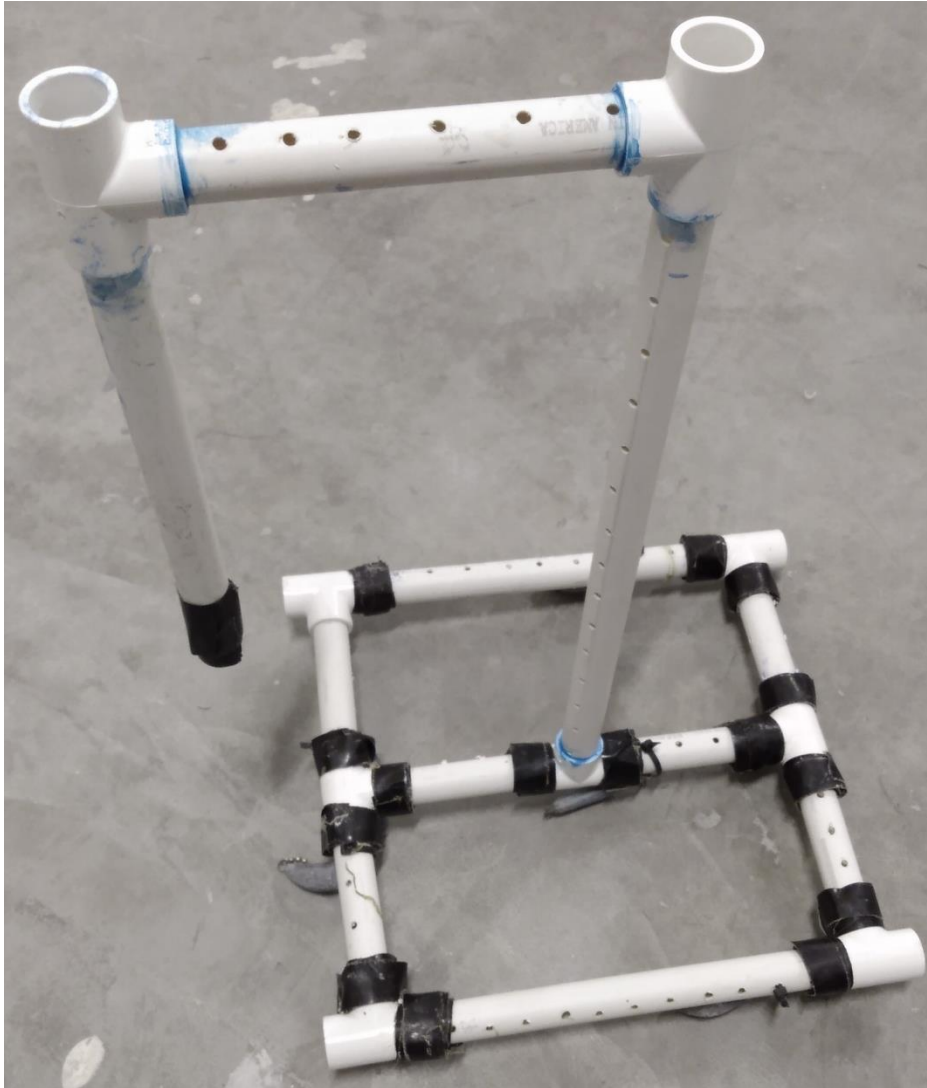
Figure S2. Support stand for the hydrophone constructed from PVC pipes and fittings. The stand is designed with holes in the PVC pipes to enable water entry, facilitating sinking. The hydrophone is suspended from the pipe at the far left.
