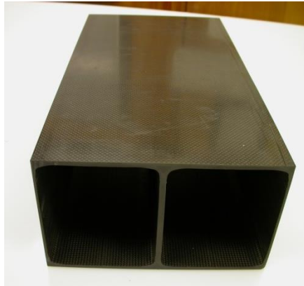
Figure 14. Representative double box beam
