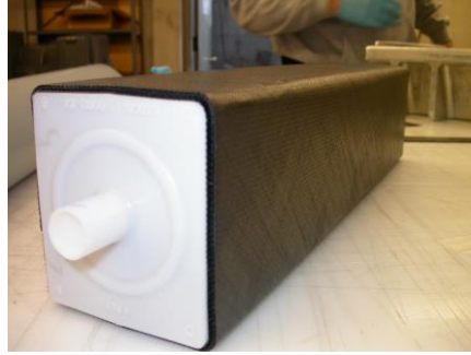
Figure 12. Image of thermoplastic cellular core with prepreg plies wrapped around
