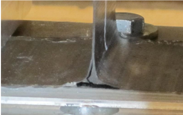
Figure 22. Image showing failure mode in cracked part at 1.5 mm extension
