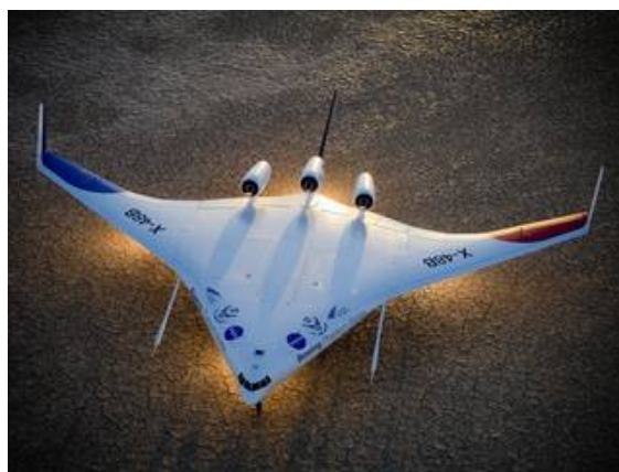
(b) Boeing's X-48B Blended Wing Body technology demonstrator. Credits: NASA Photo
