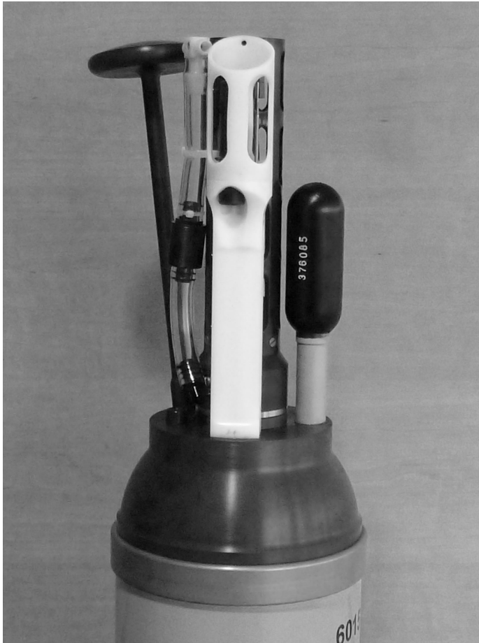
Figure 2.1. STS float endcap with both STS and SBE 41CP CTDs. Unlike the SBE 41CP, the STS unit is unpumped and does not carry a biocide.
